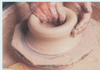
Gambar 1.22 Teknik putar ( throwing ) Sumber: Marlyn/ Midas Printing Internasional.
