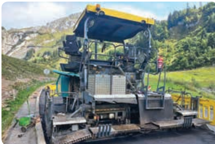
Gambar 2.14 Asphalt finisher Sumber: Asumnival/commons.wikimedia.org (2021)
