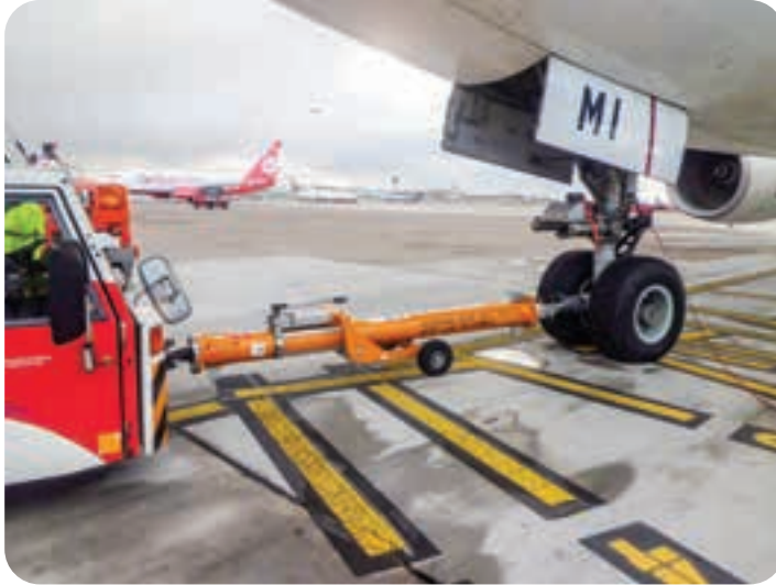
Gambar 6.90 Aircraft towing bar (Sumber: Jet Maintenance & Service, 2021)
