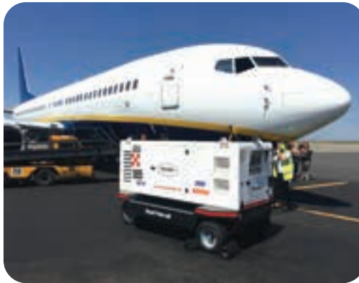
Gambar 6.88 Ground power unit saat preflight dan maintenance (Sumber: ONS Frankfurt GmbH, 2020)
