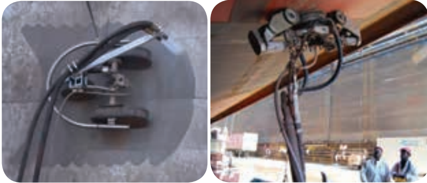
Gambar 2.19 Sandblasting Robot Mekanik
