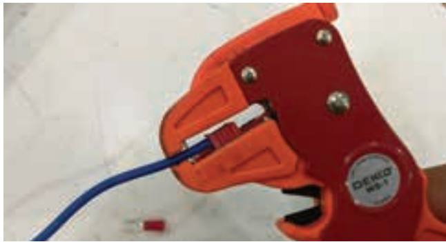
Gambar 4.33 Proses Pengupasan Kabel
