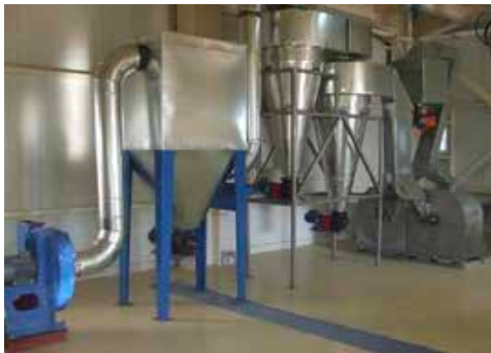
Gambar 5.13 Pengering blower ( pneumatic dryer ). Sumber: turkishexportal.com
