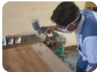
Gambar 4.69 Finishing Semprot Sumber: Suradi (2022)
