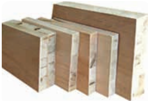
Gambar 4.55 Blockboard Sumber: Imam Damar Djati (2022)
