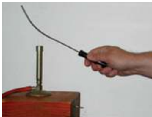
Sumber: www.physics.upenn.edu Gambar 4.6 Saat dipanaskan, bimetal melengkung.
