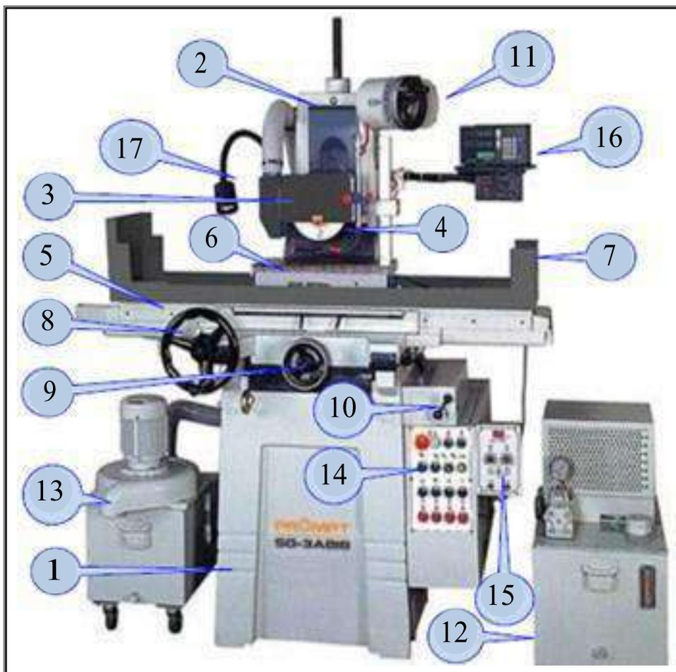
Gambar : Penampang Surface Grinding Machine Spindle Horizontal
