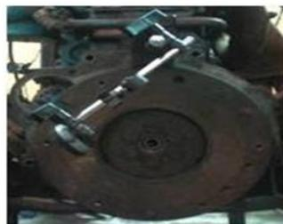
Gambar 1. Mengukur keolengan roda penerus/fly wheel
