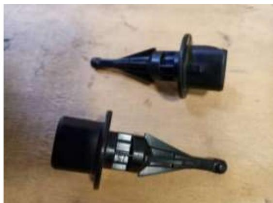
Gambar 7. Intake Air Temperature Sensor
