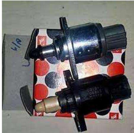
Gambar 15. Idle Speed Control
