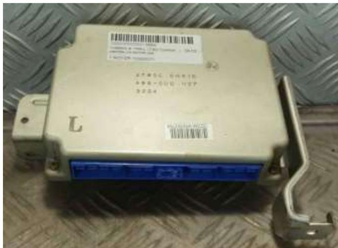
Gambar 1 Engine Control Unit
