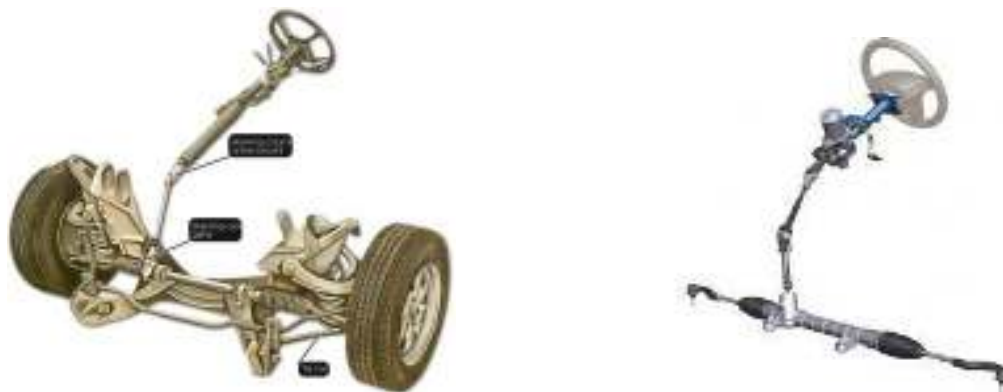
Gambar 3. Rack and pinion steering gear
