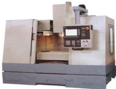
Gambar Mesin CNC Drilling & Milling
